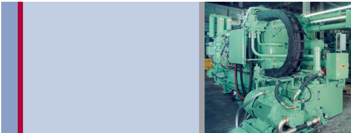
Die casting machine, pump with variable flow by speed control
